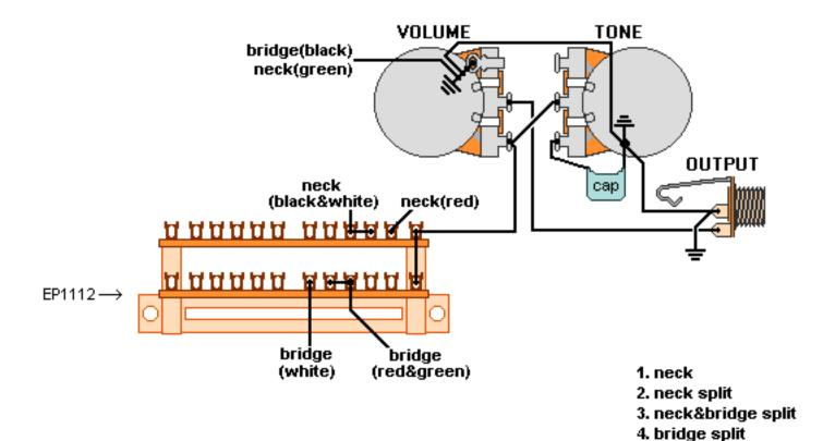
Install both pickups with cables towards controls
